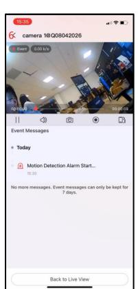
BTW: Due to the limitation of AX Pro Control Panel storage capacity, only the latest 7s video can be seen at present **Due to the limitation of host storage capacity; only the latest 7s video can be playback at present**
