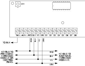
**TAM** - This can be used to tamper the cabinet the PC5208 is mounted in. Connect a normally closed (NC) switch across TAM and BLK. If the tamper is not being used connect a piece of wire across TAM and BLK to remove the trouble condition.
