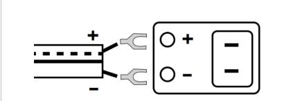
Connect power supply. WARNING! Use a 5vDC to 7vDC Power Supply ONLY
