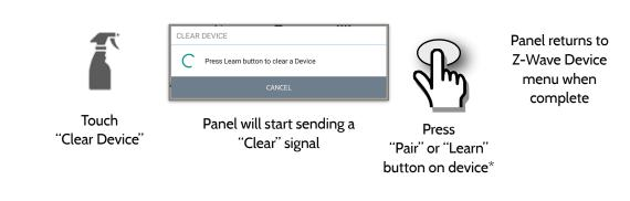
Clears Z-Wave device from a network, whether it was enrolled with another controller previously or the IQ Panel 2. Also deletes a device from the IQ Panel 2 if currently paired.
