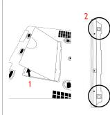
1. Insert your thumb or finger under the opening on the back cover and firmly pull up to remove. This cover is not needed for wall mount.
