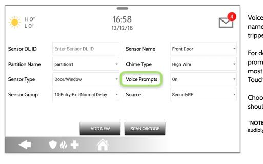
Voice prompts annunciate the sensor name when the sensor is opened or tripped.\*
