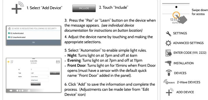
S2 is a new Z-Wave Security Protocol. When an S2 node is attempting to be included it will request S2 security keys. These are based on the level of S2 security that the end device requires. These keys can be Unauthenticated, Authenticated or Access. These keys can be manually granted by selecting the appropriate option.
