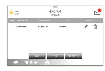
**NOTE:** The IQ Remote will automatically pair as Sensor Type "Keypad" and will appear on the zone list in the order in which it is paired. Sensor Groups 0, 1 & 2 are available options for this Sensor Type.
