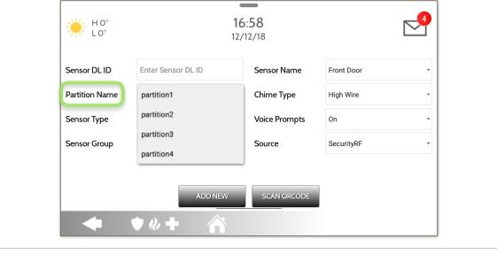
When Partitions are enabled (see Dealer/Installer Settings) you may then assign a sensor to a specific partition. This will allow independent control and arming of that partition without disrupting the main panel's master partition. You may create and use up to 4 partitions.
